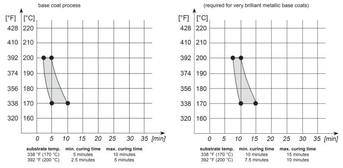
Cure parameters must be closely observed since mechanical properties will develop before full cross-linking.
